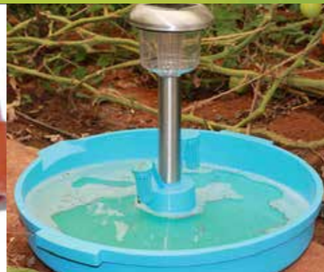
Ferolite which uses light and lures to capture Tuta absoluta moths. Farmers are encouraged to use substitutes such as modified basins with water and lure to trap moths
